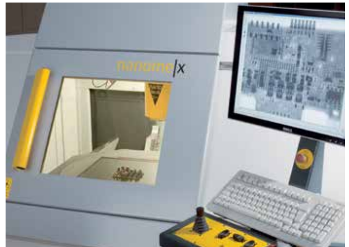
An eye that doesn't miss anything: the X-ray microscope
