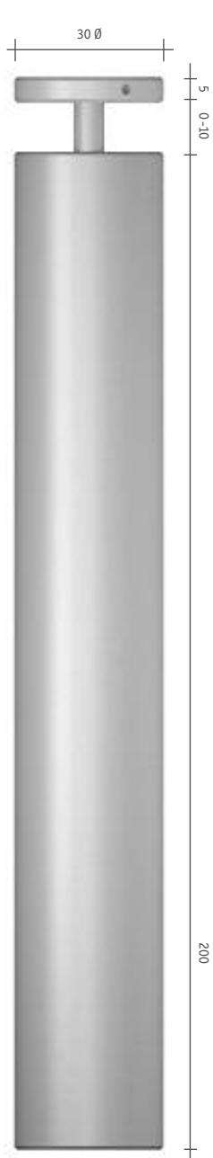
PSD.5 Panel support for drilled sheet
