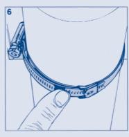
Push any remaining excess band through the buckle for a safe, tidy job. Tamtorque can be released and repositioned if required.
